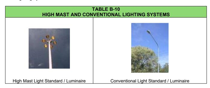
A high mast lighting system consists of steel poles ranging from 20 metres to 40 metres high. These poles support high pressure sodium luminaires. They are usually located in the centre median or within an interchange area. High mast lighting systems produce a comfortable light with minimal glare for drivers. High mast lighting is economical where many installations are required.
